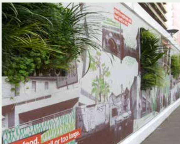
Figure 6.3: A combination of graphic image and 'green wall' may be an appropriate solution to enhance the appearance of hoarding fences.
